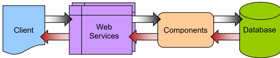
The client passes requests through HTTP or HTTPS to the MyID Data Source and MyID Process Driver web services; both services are required for full operation. The web services communicate using DCOM with the MyID components on the application server; these components provide the business logic and communicate with the MyID database. Responses are returned to the client through the MyID web services.
